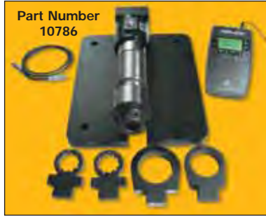
RCA-3000 Torque Range 300-3000ft/lb Accuracy +/- .25%
